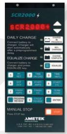
to delay gassing from 1-8 hours. If during your workday, the battery is never on charge for more than one hour, simply set the delay for one hour. If a connected battery reaches the gassing voltage within one hour, the charger will suspend charging. At the end of the delay time, the charger will resume its normal charge routine, taking the battery through the essential gassing portion and finish charge the battery.
