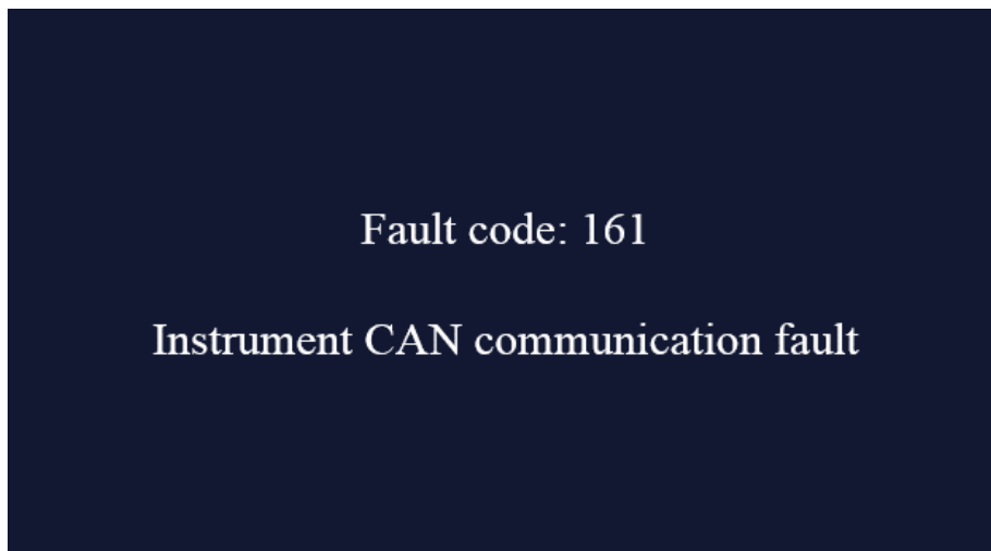
Fig. 4-5 Instrument interface-fault display
