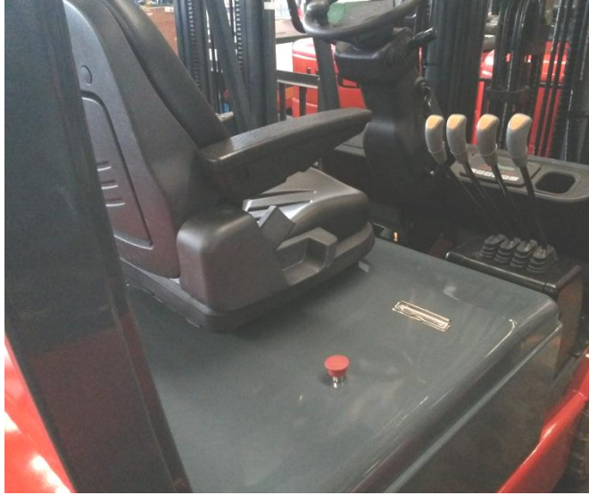
Figure 4-7 Emergency power off device
