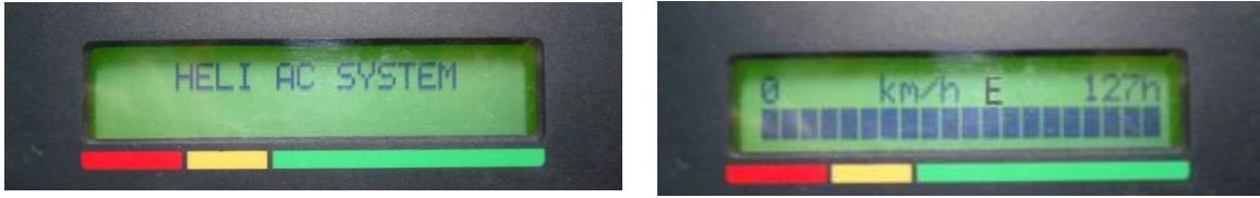
Fig. 4-19 Display interface on the ZAPI instrument (no fault)
