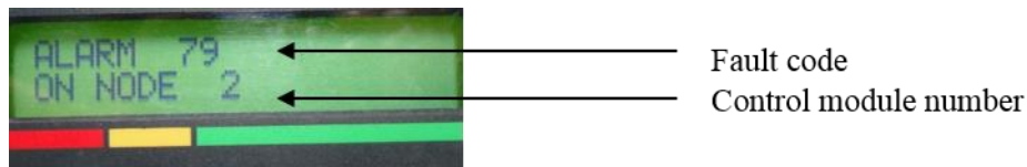
Fig. 4-20 ZAPI instrument fault display interface
