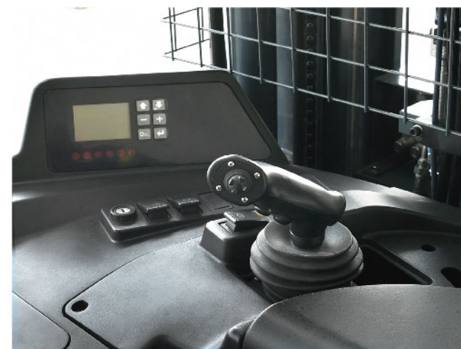
Multi-function joystick handle and proportional controls produce are easy and intuitive to use
