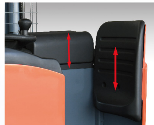
Adjustable backrest and armrest help reduce fatigue
