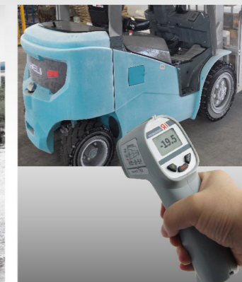
The whole vehicle can be operated alternately in -20°C cold storage for 6 hours and parked in the cold storage for 12 hours without any failure and can continue to work.
