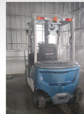
IPX4 waterproof: the vehicle is powered on to simulate a 15min short-time 5000L rainstorm test, and the vehicle can continue to run without failures.
